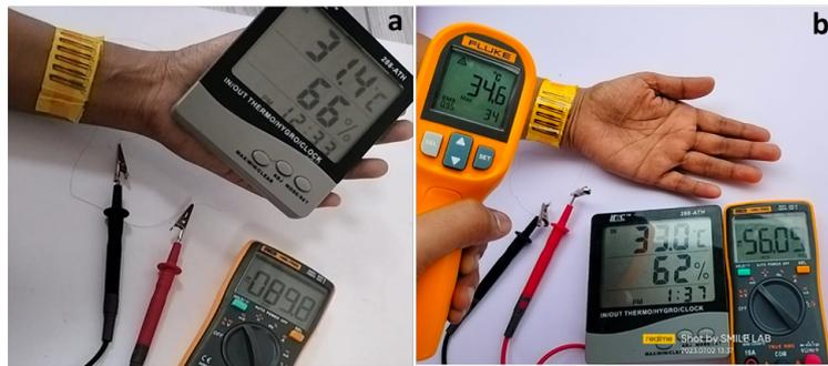
Figure 12: Wrist wearing PN type FTEG a) Indoor ambient b) Outdoor environment
