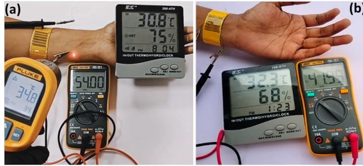
Figure 11: Wrist wearing Pi type FTEG a) Indoor ambient b) Outdoor environment
